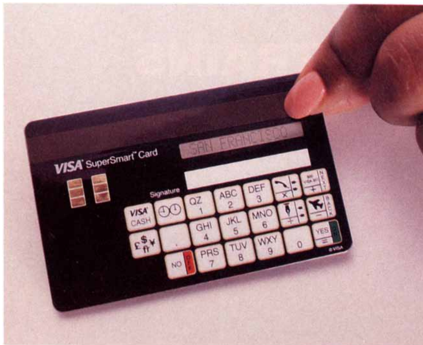
COMPUTERIZED CREDIT CARD developed by Toshiba and Visa International contains a microprocessor, memory, keypad and display. Although this card identifies its user during transactions, the same hardware could be reprogrammed as a personal representative for spending digital cash.
